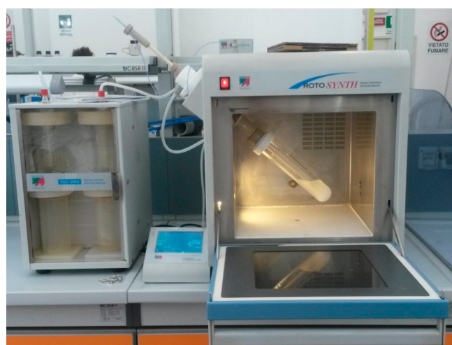
Figure 1. MW-reactor Rotosynth (Milestone srl, MLS GmbH).
